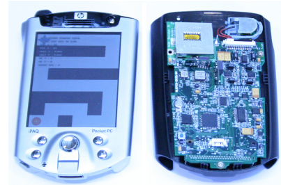
Figure 1. MESH hardware shown next to an iPaq running a simple tilt-driven maze game
